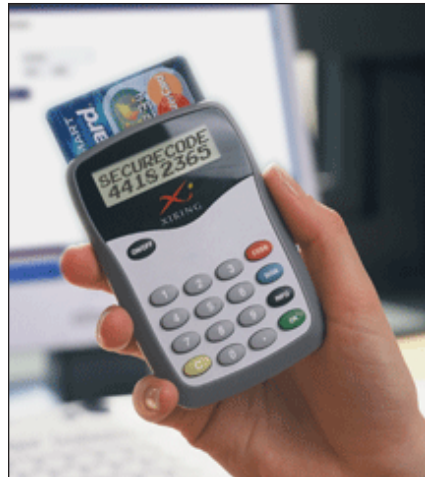
Figure 25: A one-time password calculator. (Photo source: www.reseaux-telecoms.net 37 )
