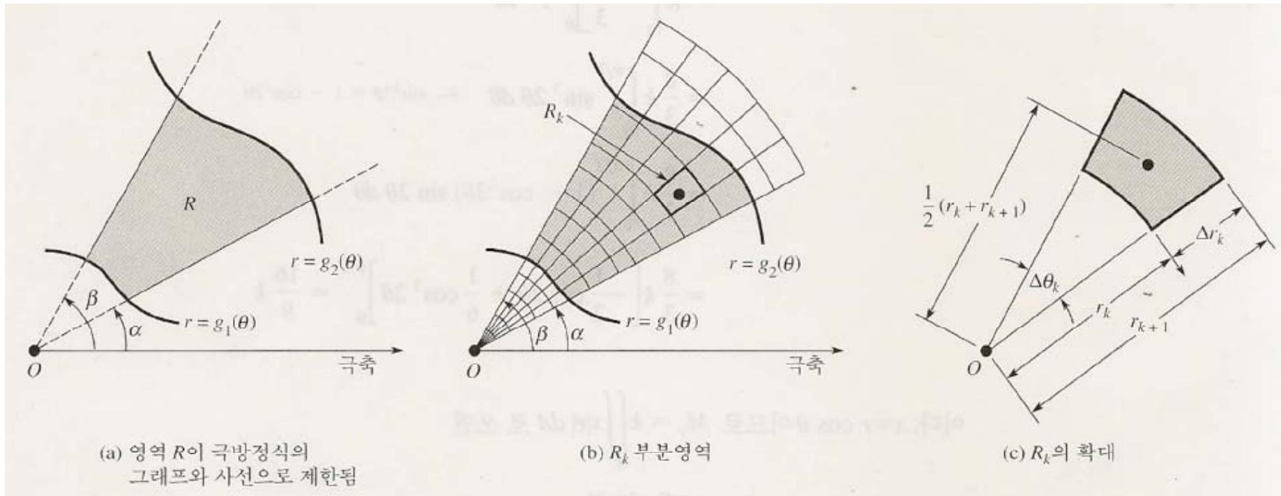
$$\Delta A_k = \frac{1}{2}(r_{k+1}^2 - r_k^2)\Delta\theta_k = \frac{1}{2}(r_{k+1} + r_k)(r_{k+1} - r_k)\Delta\theta_k = r_k^* \Delta r_k \Delta\theta_k$$
